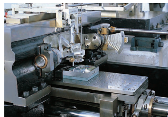
Ruling engine used to fabricate diffraction gratings
