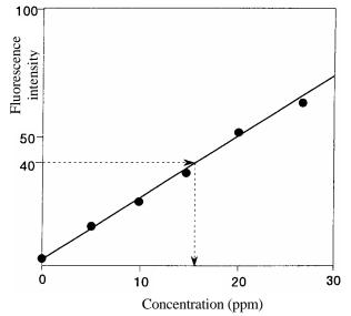
For example, suppose the fluorescence intensity of the specimen is 40. By consulting the calibration curve shown in the right-hand figure, the concentration of the specimen can be estimated at 16 ppm.
