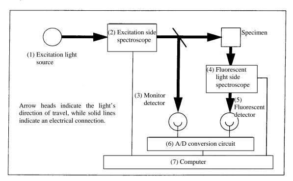
White light (light composed of various wavelengths) emitted from the light source enters an excitation side spectroscope (2). While measuring an excitation spectrum, this excitation side spectroscope (2) is moved to successively change the wavelength used to irradiate the specimen (this is called scanning or wavelength scanning). In contrast, when measuring a fluorescence spectrum, a specific wavelength is selected and fixed in the excitation side spectroscope.
