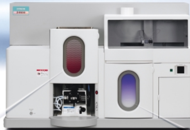
Z-2000 TANDEM TYPE ATOMIC ABSORPTION SPECTROPHOTOMETER
